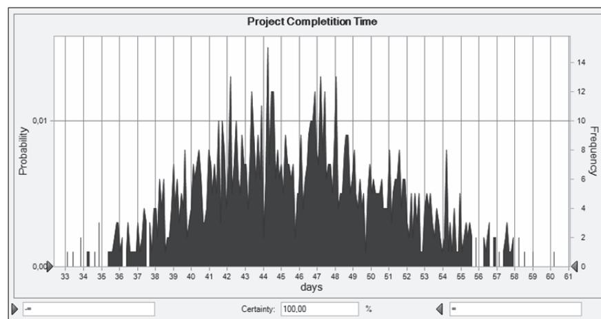
Figure 3: Frequency chart for project completion time
