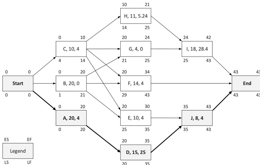
Figure 1: The “activity-on-node” network diagram for selected project
